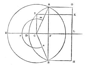
Let ADB be a parabolic reflector and C its focus, then will DC be the minimum and AC the maximum focal distance. Now if the light at C emanated from a point, all the rays intercepted by the surface ADB would be projected forward in parallel lines and cover the plane surface GH = AB at whatever distance it might be placed
